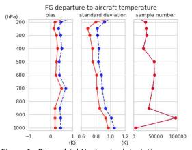
Figure 1. Biases (right), standard deviations (center) and sample numbers (left) of fits of the first-guess departure to aircraft temperature data in the experiment. Blue: noBC; red: BC.
