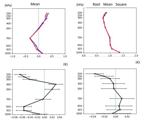
Figure 3. Fits to radiosonde data for 12-hour forecasting of temperature in the experiments. (a) Vertical profile of mean error (ME), (b) BC-noBC of ME, (c) vertical profile of root mean square error (RMSE), (d) ratio of RMSE change ((BC-noBC)/|noBC|). The red and blue lines represent BC and noBC, respectively, and error bars represent 95% confidence intervals.
