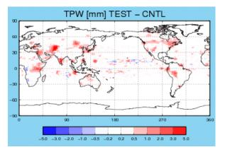
Figure 3: Average differences in analyzed values of PW between the control (without GPS-PW) and the test (with GPS-PW). The sampling period was from August 1 to August 31, 2010.
