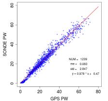
Figure 1: Scatter plots of GPS-PW data against sonde-PW values. The sampling period was from August 1 to August 31, 2010. The red line represents the linear regression derived from the scatter plots.
