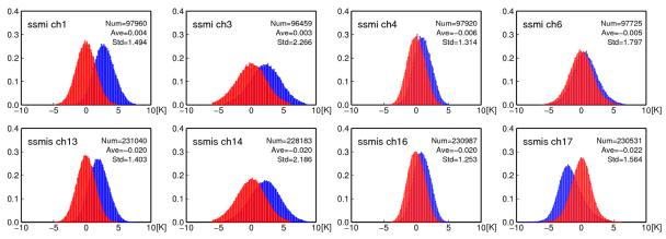
Figure 1. O-B statistics for DMSP-F13/SSM/I (ch. 1, 3, 4, 6) and DMSP-F16/17/SSMIS (ch. 13, 14, 16, 17). The red histogram areas are for after air-mass bias correction, and the blue ones are for before.
