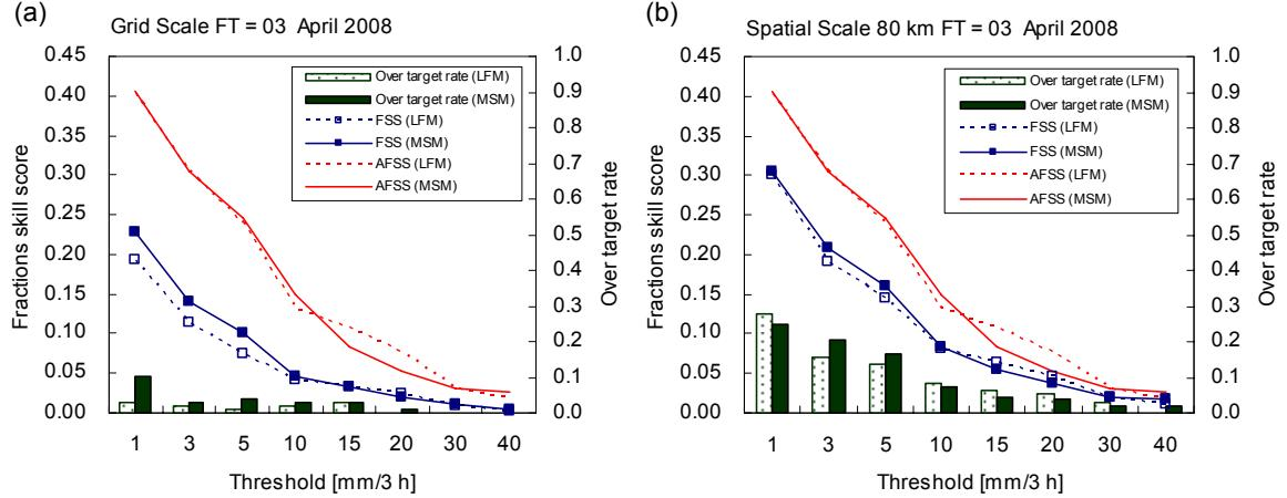
Figure 1. Fractions skill score (line plots with symbols), asymptotic fractions skill score (line plots) and rate of over-target skill (bar charts) are shown as a function of threshold and three hour accumulation. Each score was calculated in (a) the grid scale, and (b) the spatial scale of 80 km.
